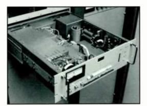
All exciter components are easily reached from the front of the transmitter. Exciter moves on tracks for easy access; shown here with top cover
